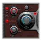
To use the noise generator, you first need to turn it on. This can be done with the On/Off button. When in an active state, the button is red.
