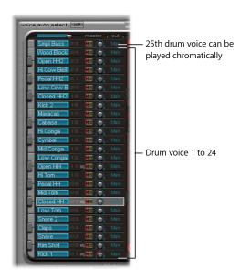
You can compare Ultrabeat to a drum machine that features 24 drum pads plus a built-in keyboard.
