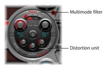
The order that sounds are passed through the filter and distortion unit is determined by the arrow found at the "equator" of the Filter section. Clicking the arrow switches between the arrow up (distortion, then filter) and arrow down (filter, then distortion) settings.
